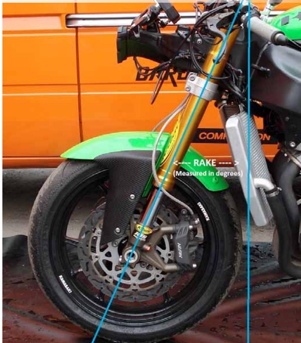
» 3. The trail is the distance on the ground between the centre of the tyres contact patch and the point where the centre line of the forks intersects the ground.
