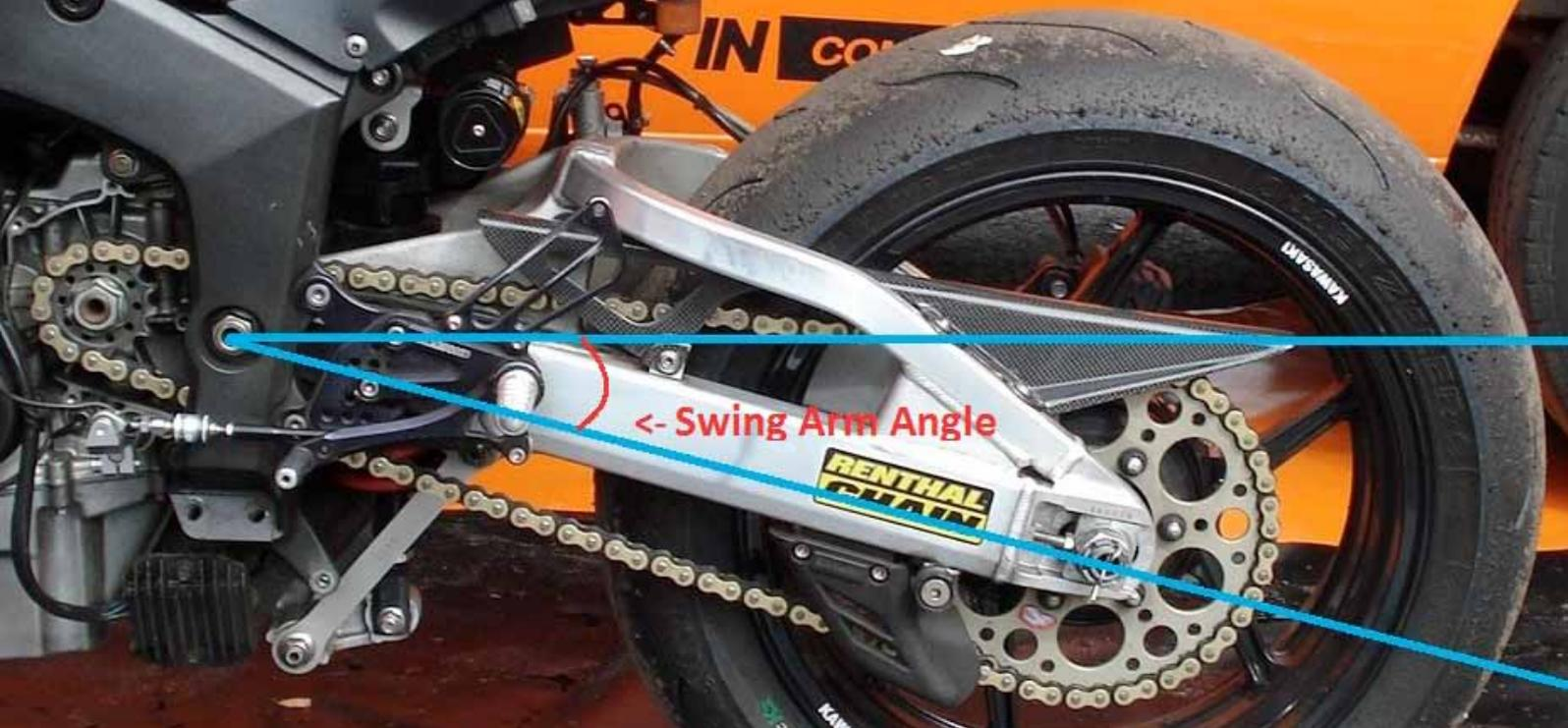
» 4. The Swing Arm Angle is the angle between a line drawn parallel with the ground and the line through the swing arm pivot and read wheel spindle.
